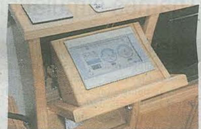
The cunningly hidden touch screen used to access the boat monitoring system.
